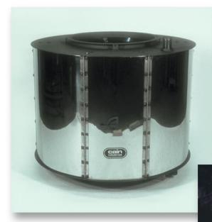
The FCR Series is a more custom designed heat exchanger which can be applied in cold water condensing heat exchangers, confined area restrictions, and is offered in stainless, carbon, or Al-Fuse fin tubing. Flexibility allows specific engineering requirements to be met such as fin spacing for fouling conditions and low gas pressure drops.
