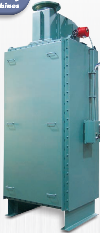
Innovative Energy Systems , Oakfield, New York (7) Model HRSR-330C26SSP Recovering 1,845,000 Btu/hr each from (7) Caterpillar 3516 engine. Reducing each 922°F to 387°F @ 2,766 SCFM; Raising 300 GPM hot water from 180°F to 194°F.
