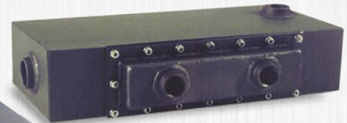
Mobile Trailer , Venice, California Model UTR-630218CSS. Recovering Btu from a 33kW natural gas engine. Reducing 1,282°F @ 76 SCFM to 319°F; Raising 27 GPM 50% ethylene glycol from 190°F to 198°F
