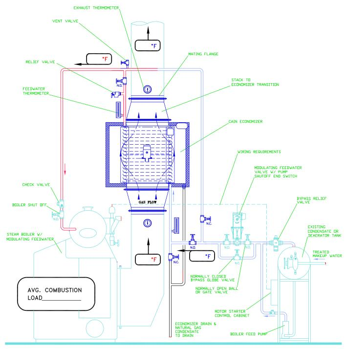
THIS FLOW DIAGRAM SUGGESTS A BASIC FLOW DESIGN AVAILABLE FOR CONSIDERATION REGARDING THE INSTALLATION OF A CAIN EXHAUST STACK ECONOMIZER. AS IT MAY BE MODIFIED DEPENDING ON SPECIFIC INSTALLATION REQUIREMENTS OR AN ALTERNATE FLOW DESIGN WHICH MAY BE REQUIRED, CAIN INDUSTRIES IS NOT RESPONSIBLE FOR ANY MODIFICATIONS, CHANGES, OR SELECTIONS.
